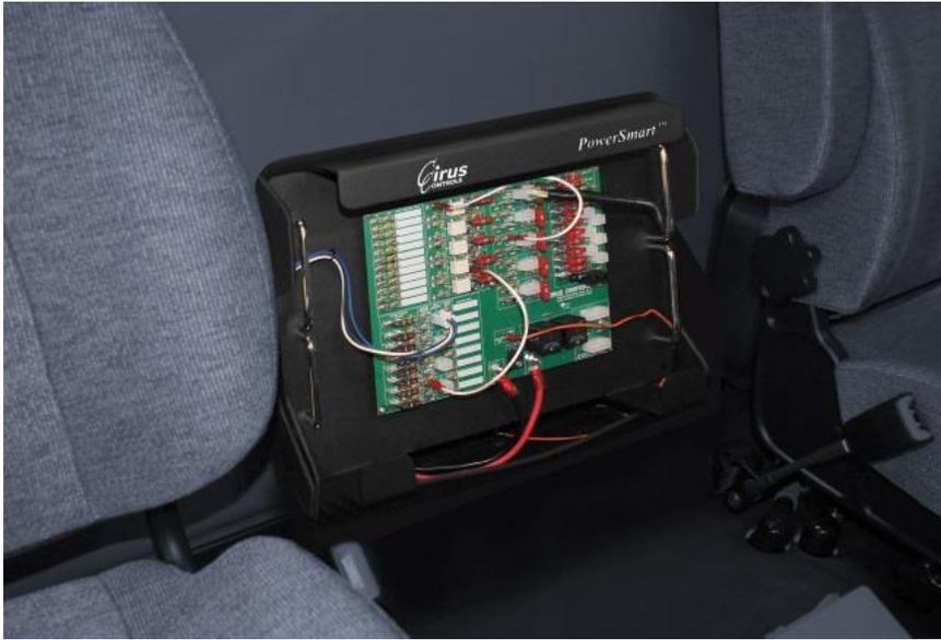
The PowerSmart installed in a snowplow truck.
