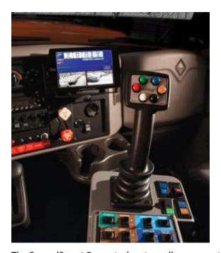
The SpreadSmart Rx control system allows operators effortless control of salt applications while logging data on application rates, location and speed.
