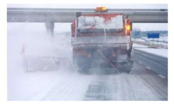
An Iowa Department of Transportation truck plows a highway lane while using a SpreadSmart system from Cirus Controls to precisely meter salt onto the roadway and upload speed and location data for real time or later analysis.
