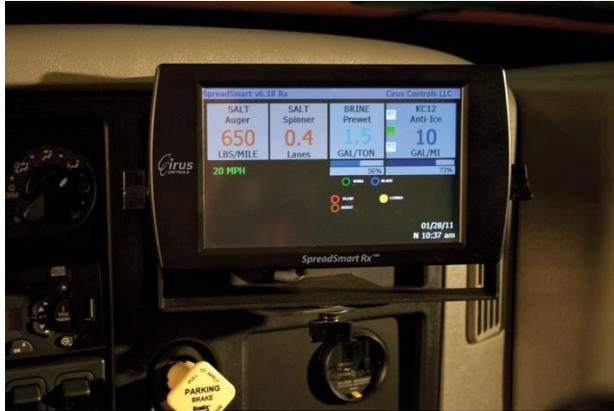
SpreadSmart Rx spreader control systems offer numerous mounting options including a dashboard display.
