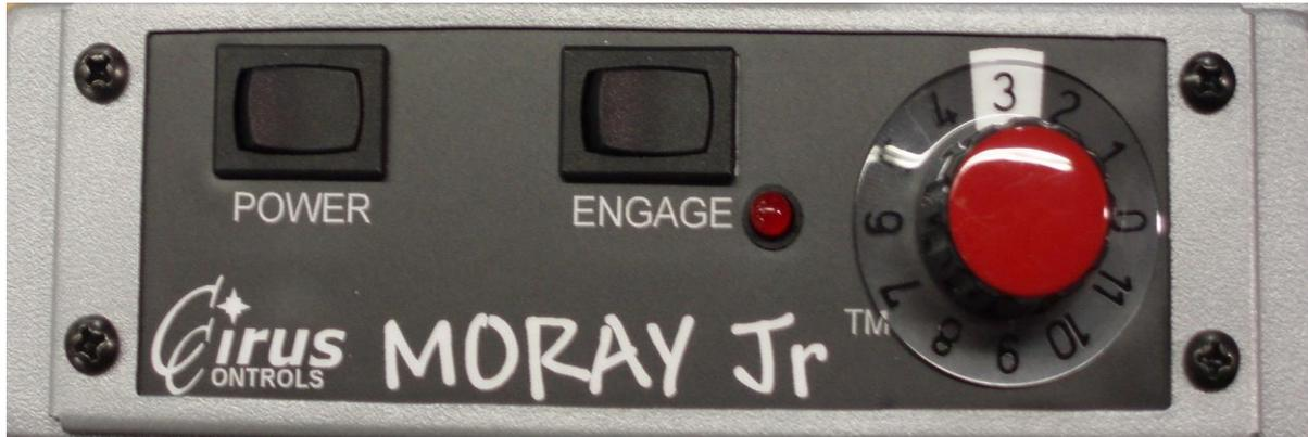
**Power Switch:** Main system power switch.
