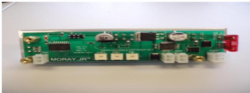
**POWER:** Provides power and ground to unit. (MK-1003 cable)
