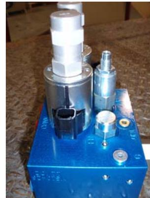
**Coil Mounting:** coils are held in place by a single nut from the top that must not be tightened more than 20 ft. lbs. **Nominal torque settings are 10-12 ft. lbs. Over tightening can damage the coil or the valve stem underneath.**
