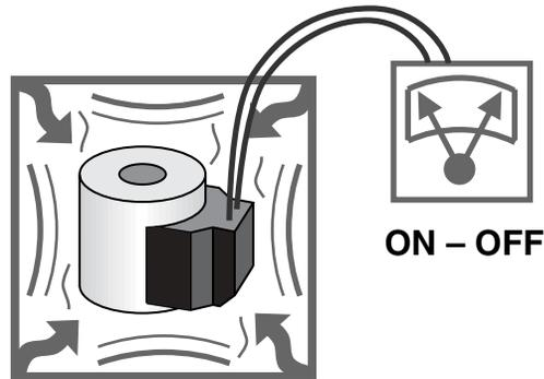
**This accelerated test simulates temperature cycling to induce cracks or separation between components of the coil.**
