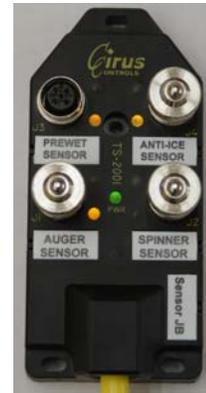
With pigtailed removed, presence of amber LED confirms NPN setup and good harness wiring;
