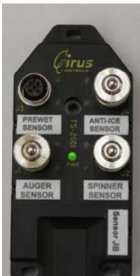
Power is on, one NPN sensor enabled
