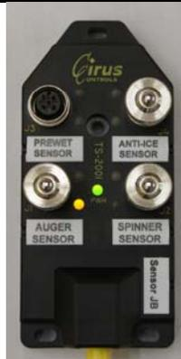
Power is on, three NPN sensors enabled
