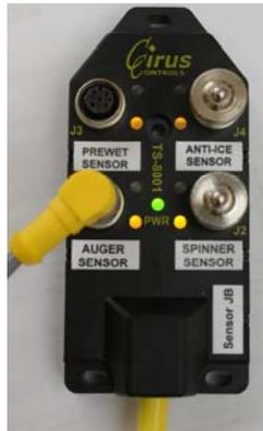
Steady amber LED may indicate sensor stopped at gear tooth; Remove pigtail or rotate device to confirm;
