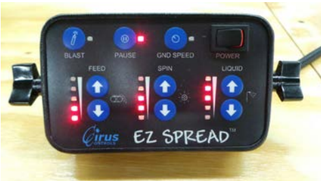
Pause LED On (spreading paused) Feed LED=2, Spin= 4; Liq=6
