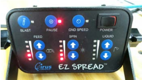
Pause LED On, Spreading stopped
