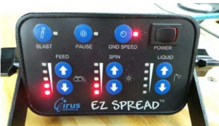
GND LED On constant, spread normal Ground speed oriented.
