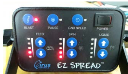
Blast LED On, Blast spreading 10 seconds
