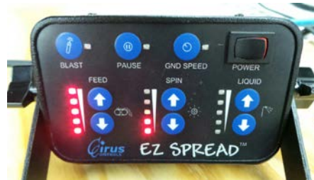
Pause LED on (spreading paused) Feed LED=10, Spin= 4; Liq=0
