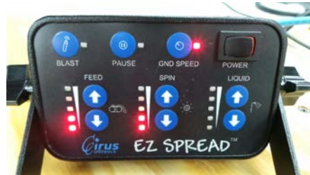
If top feed, spin, or aux led is flashing, an open Or shorted hydraulic circuit is detected.
